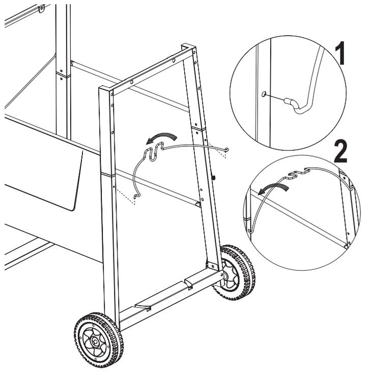
**7** Attach LP Gas Tank Block Wire
